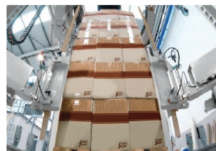
○ ACBA: Automatic Corner Board Application
